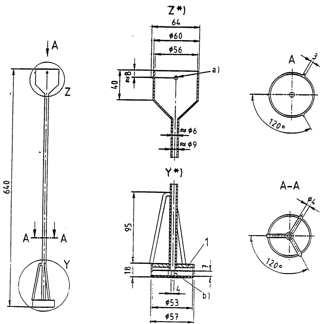
1 sintered glass filter (porosity P 160)
